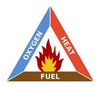
Fire fighting equipment works by removing one of the three elements of the fire triangle, for example fire blankets cut off the oxygen supply. Fire prevention means stopping the elements getting together in the first place. Removing oxygen from the environment is impossible as it is necessary for life, but heat and fuel, although always present, are controllable.
